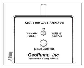
The Model 5750 Shallow Well Sampler is a portable, peristaltic pump with a maximum lift capability of 26 feet. This pump is ideal for purging shallow monitoring wells, cleaning GeoPump bladder pumps and tubing assemblies and a variety of applications where it is necessary to move small volumes of liquid.
