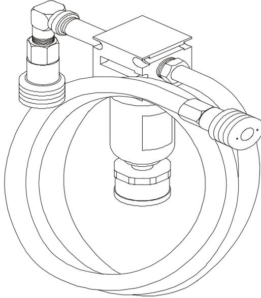
**25 Foot Long Controller To Air Supply** – Includes Moisture Trap Filter
